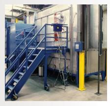
In addition to saving energy, continuous batching promised to simplify powder application: The conveyor could halt loads of parts in the powder enclosure and give the applicators more time with the parts. This would allow the applicators to inspect the coating thoroughly...
