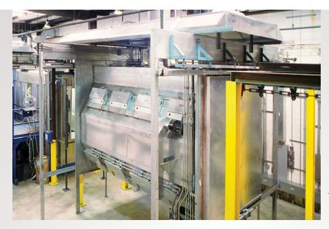
Victor Stanley's coating system uses two ovens and twice the powder of most coating systems. Be that as it may, Jerry Skalka, company vice president, pointed out that the system wasn't designed to skimp on powder. It was designed to improve quality.
