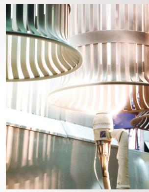
in succession, the company calls it a continuous batch system. In addition to saving energy, continuous batching promised to simplify powder application: The conveyor could halt loads of parts in the powder enclosure and give the applicators more time with the parts. This would allow the applicators to inspect the coating thoroughly before the parts entered the cure oven, which would reduce rework. The next concern was how to apply powder to the hot surfaces.
