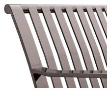
RB-28 bench detail: furniture-quality finish joints,  $1/4 \times 1-1/2$ in (6.4 x 38 mm) vertical solid steel seat ribbons,  $1/2 \times 2$  in (13 x 51 mm) solid steel arm frames for comfort and support.
